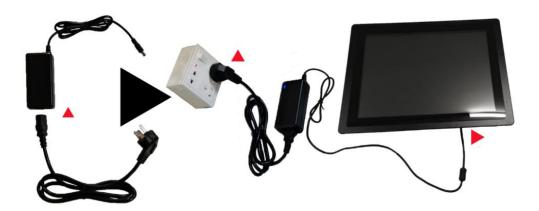
1. If the machine is not set to power on, press the "POWER" key switch after connecting the power supply.
